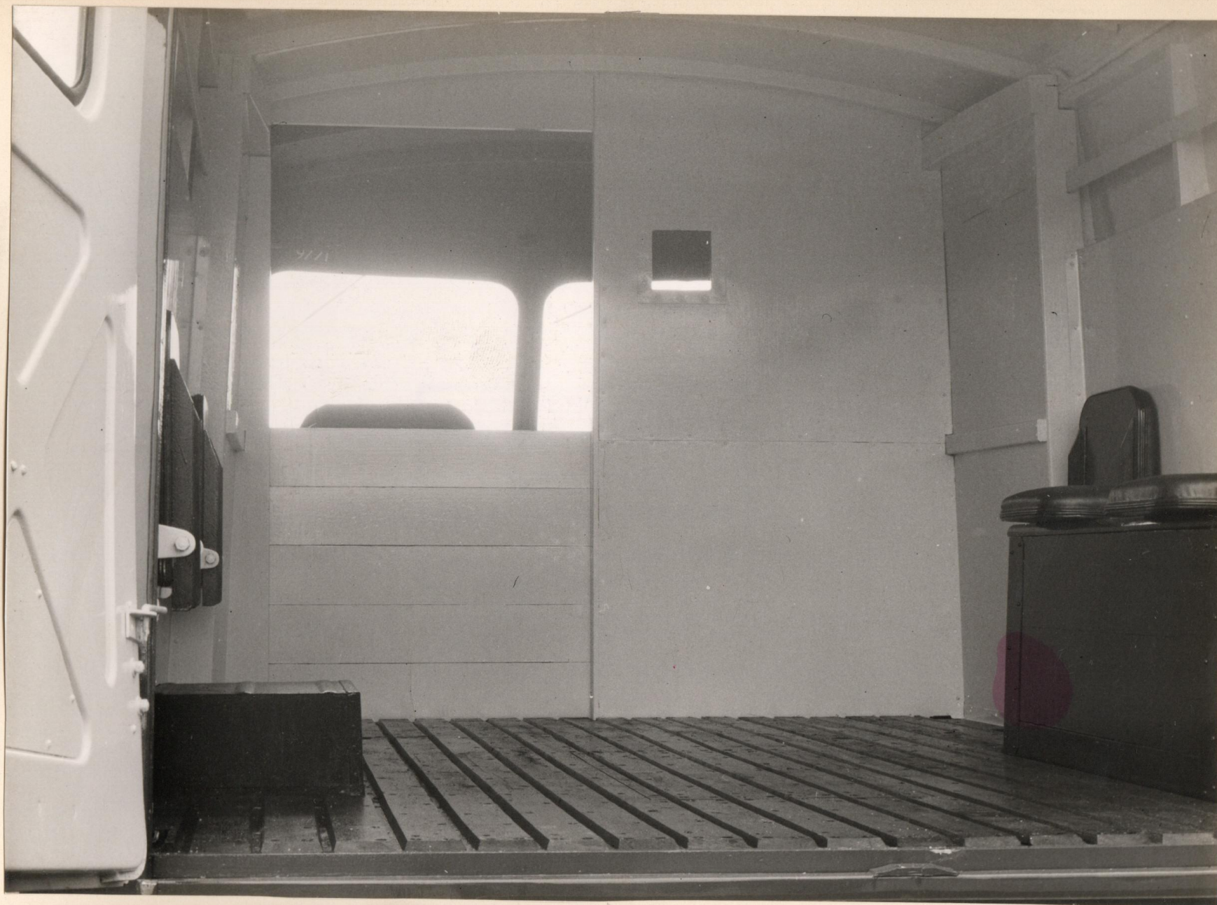
1048AS~INTERIOR VIEW SHOWING REMOVABLE \frac{1}{2} BULKHEAD.
