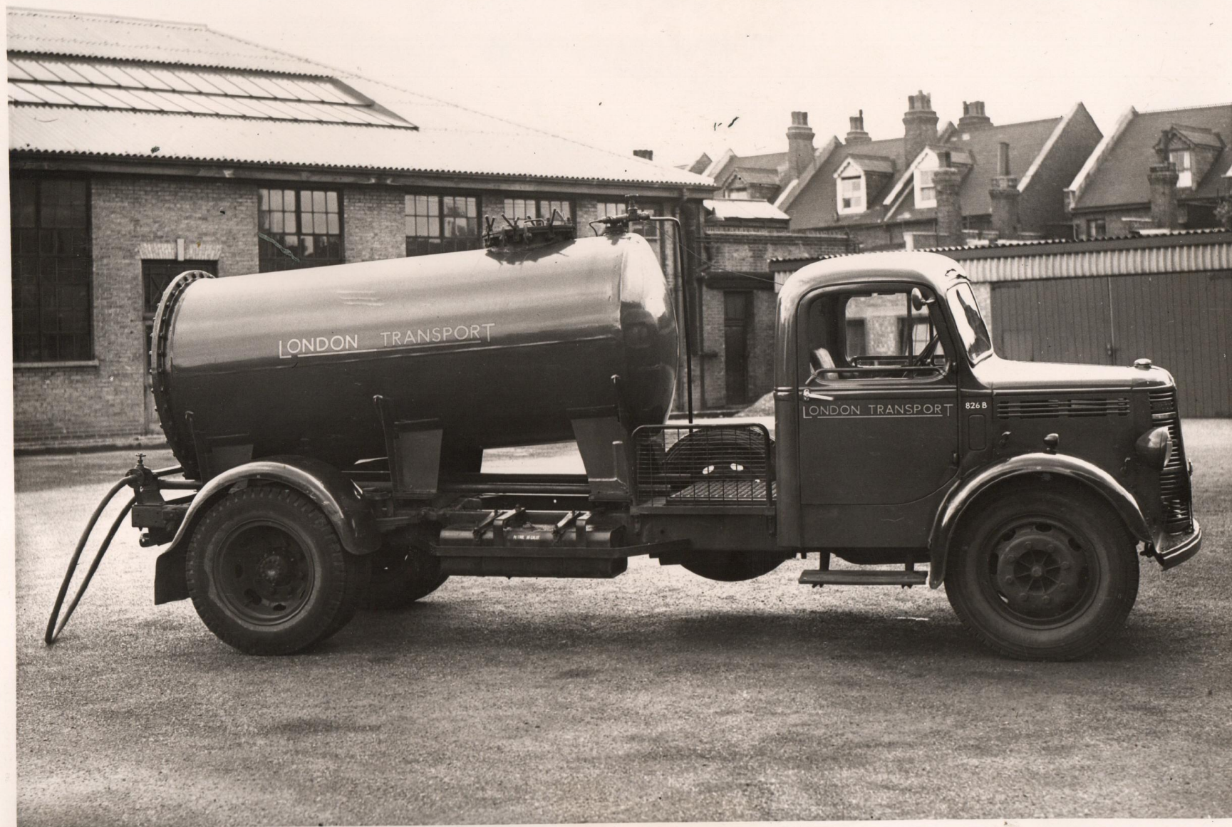
OFF SIDE VIEW 5 TON BEDFORD DISTILLED WATER TANKER. TANK REMOVED FROM ALBION CHASSIS
