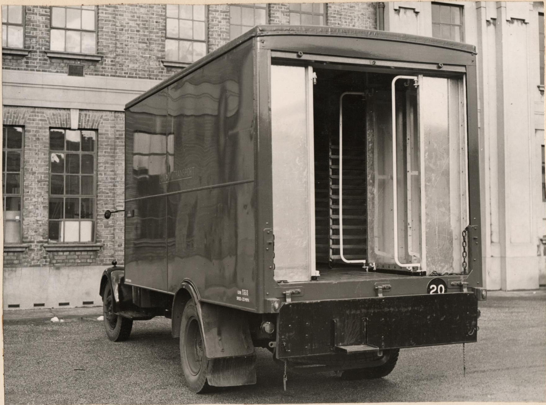
697B 5TON BEDFORD SHEWING MEAT & FISH COMPARTMENT
