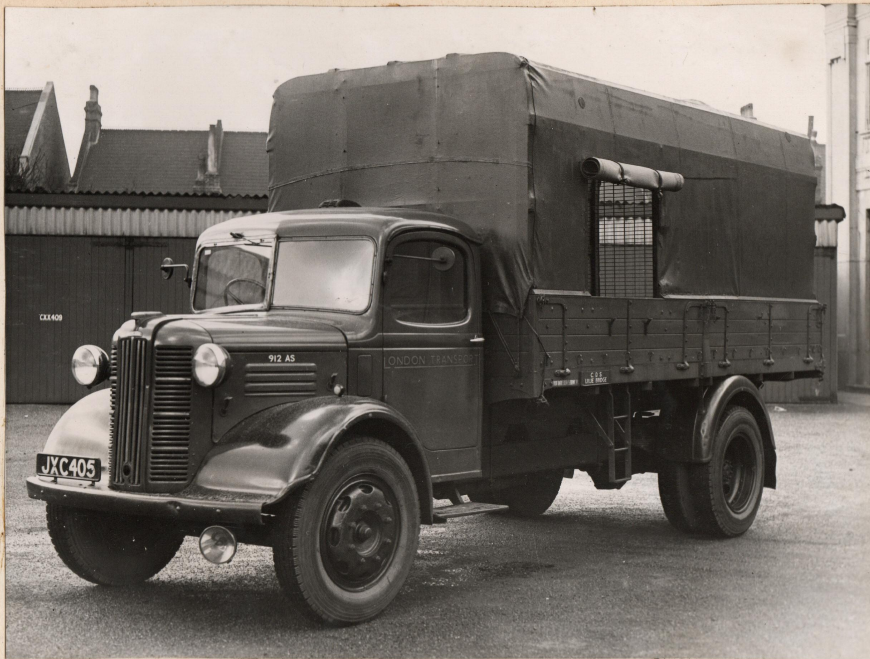
912AS 5TON AUSTIN LORRY MODIFIED FOR CARRIAGE OF STATION STORES 3/4 N/S FRONT VIEW
