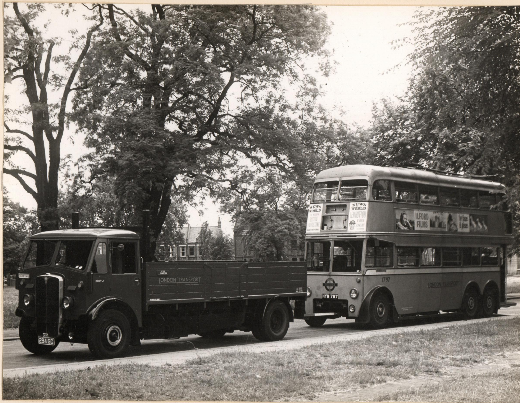
1009J 7TON A E C REGENT (CONVERTED BUS CHASSIS) TOWING TROLLEYBUS
