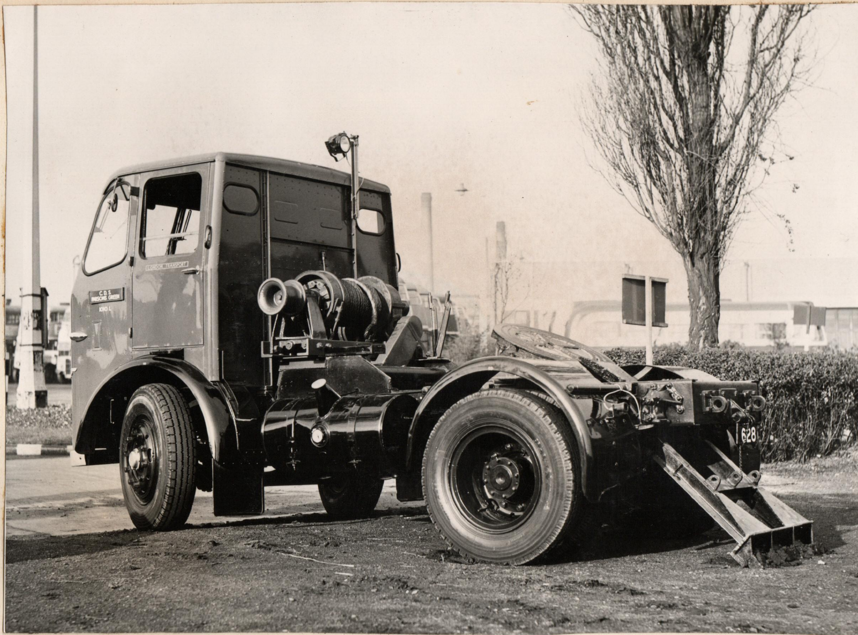
LEYLAND "BEAVER" TRACTOR UNIT 1010 L SHOWING GROUND ANCHORS IN USE.
