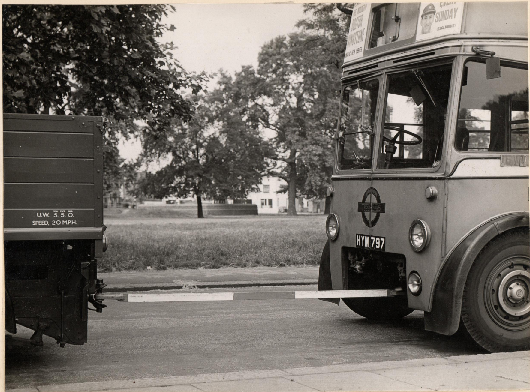
1009J SHEWING ARRANGEMENT OF RIGID TOWING BAR
