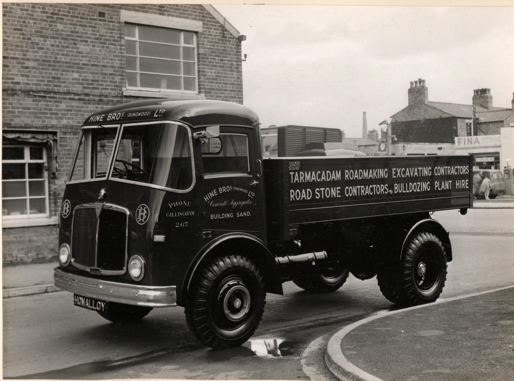
FIBRE GLASS CAB AND ALLOY BODY.
