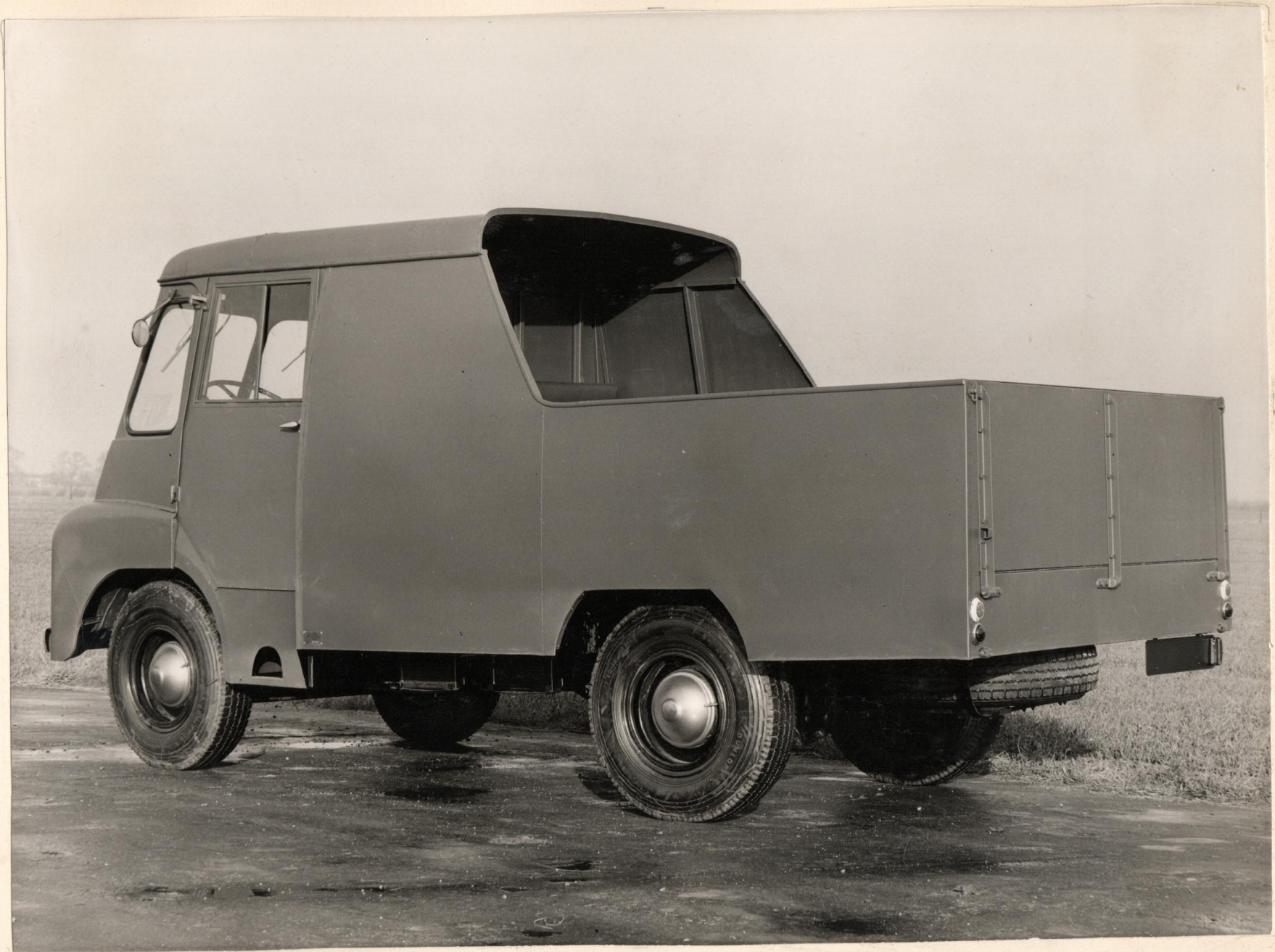
30 CWT AUSTIN TRUCK SPECIAL BODY MADE BY MARSHALL MOTOR BODIES CAMBRIDGE
