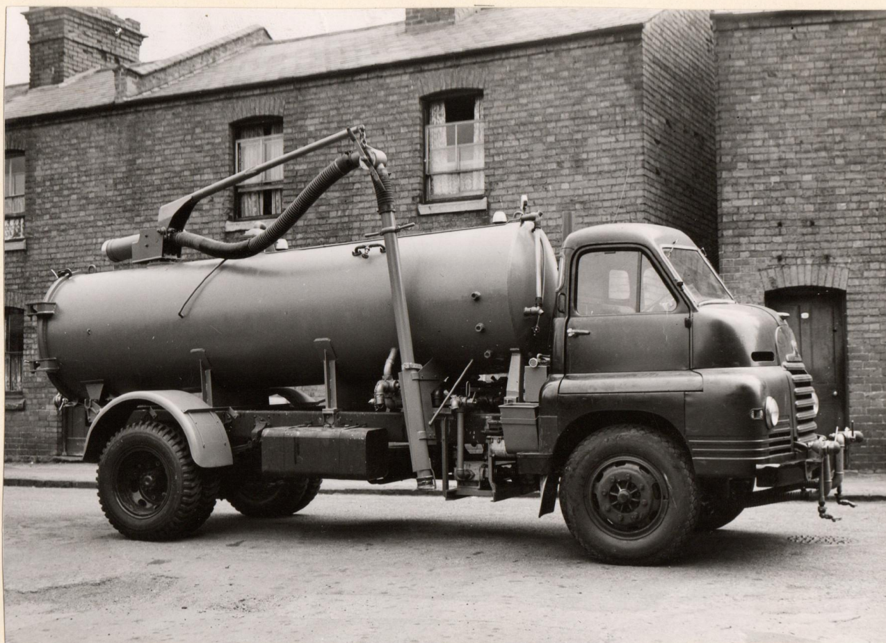
EAGLE GULLY EMPTIER SUPPLIED TO SWITZERLAND BEDFORD 'S' TYPE CHASSIS
